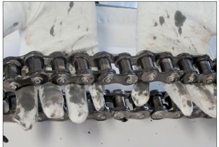
The solid white lubricant formulation (left) of Klüberfood NH1 CH 6-120 SUPREME is NSF H1 registered for incidental contact, providing a food-grade solution for chain lubrication at extreme temperatures without the residue of typical lubricants (right).
